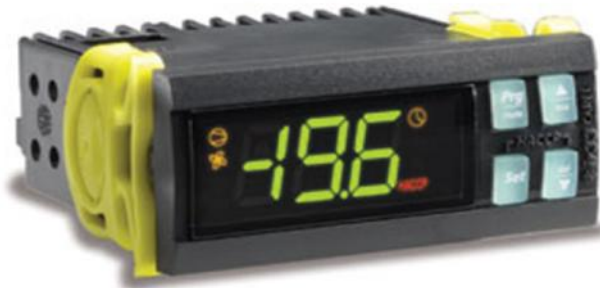
Panel mounting by two lateral sliding plastic brackets
